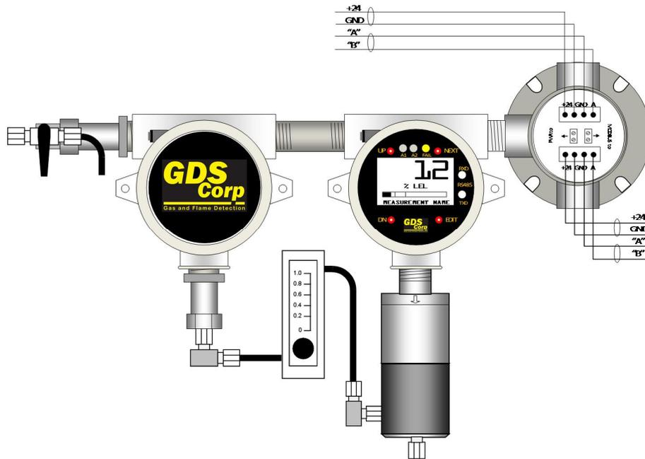
Figure 5-8: GDS-58XP with MODBUS Wiring Junction Box [MBJB]
