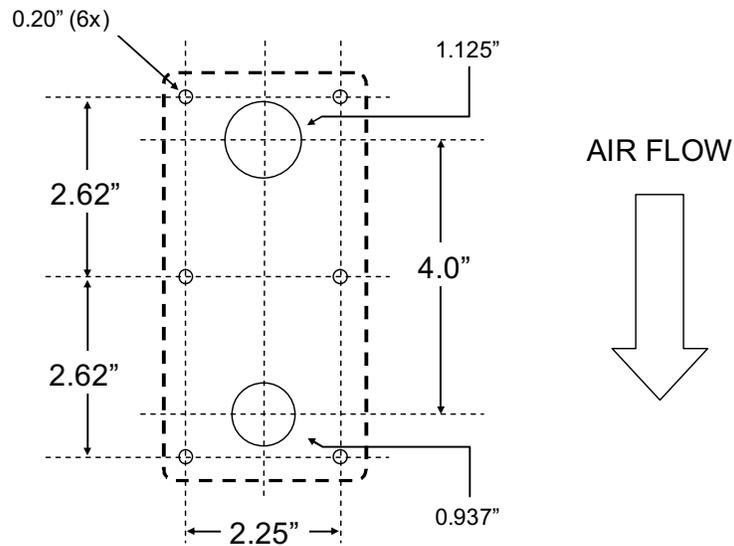
Figure 15-2: Sample Draw Duct Assembly Hole Mounting Pattern
