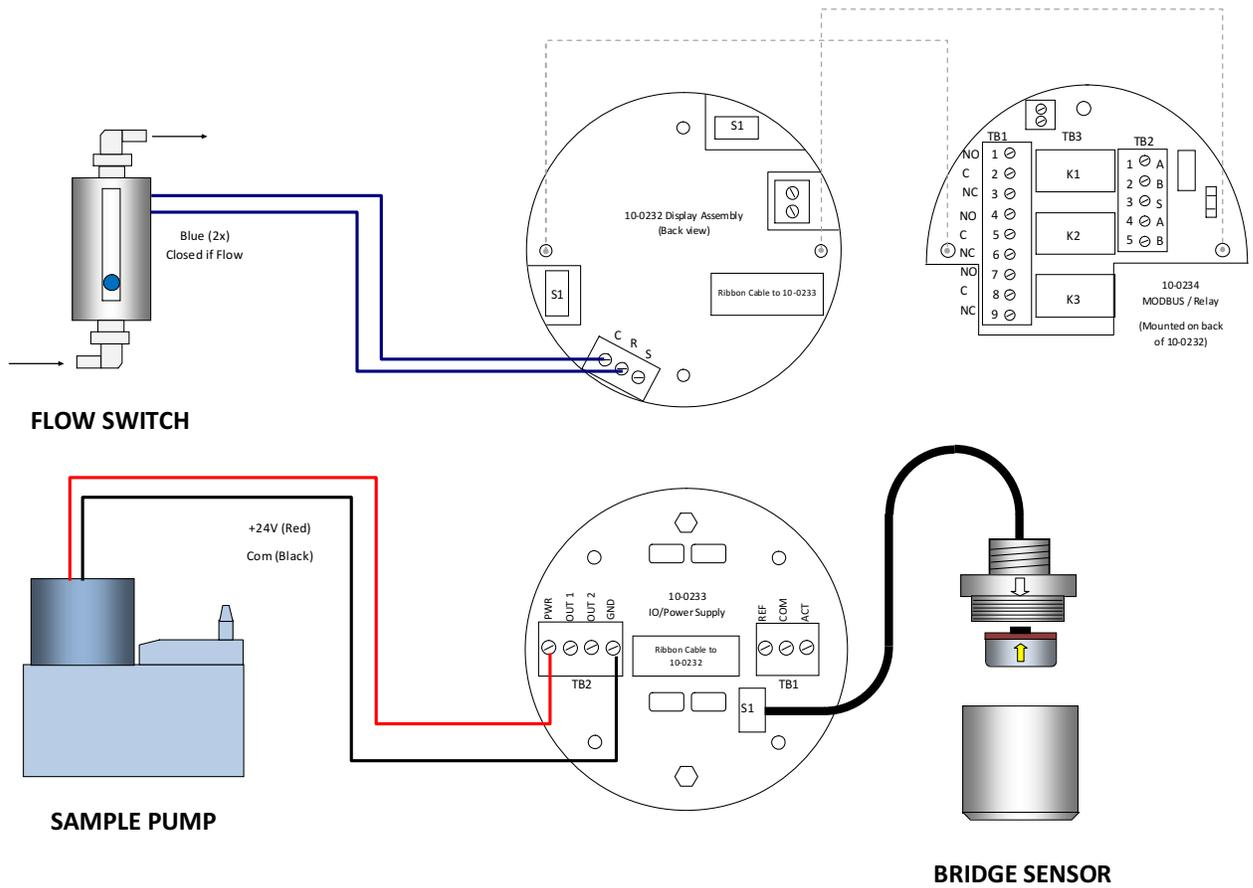
Figure 14-2: GDS-58XP Wiring Diagram (Bridge Sensor)
