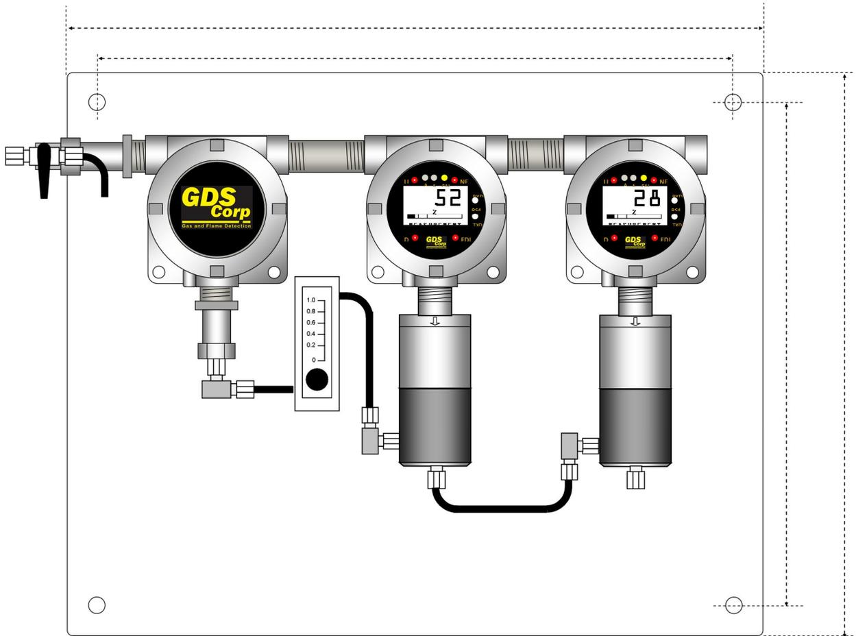
Figure 13-5: GDS-58XP 21'' x 17'' Mounting Plate Dimensions (SS Enclosures)
