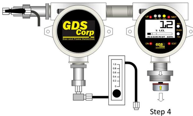
Step 4: Pulling straight down, remove the existing sensor.
