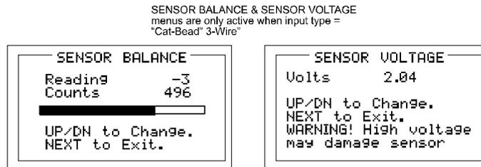
**Figure 9-3: Sensor Balance & Voltage Set Menu**
