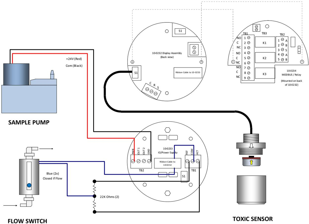
Figure 14-1: GDS-58XP Wiring Diagram (Toxic Sensor)
