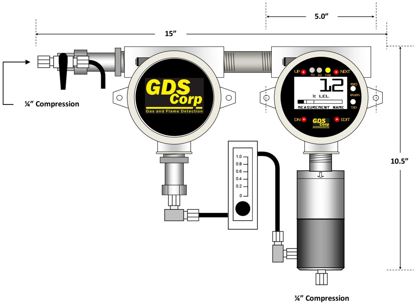
Figure 13-1: GDS-58XP Dimensions (Aluminum Enclosure)
