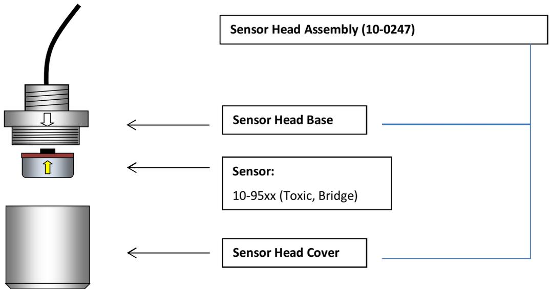
Figure 12-2: GDS-58XP Standard Sensor Head Exploded View
