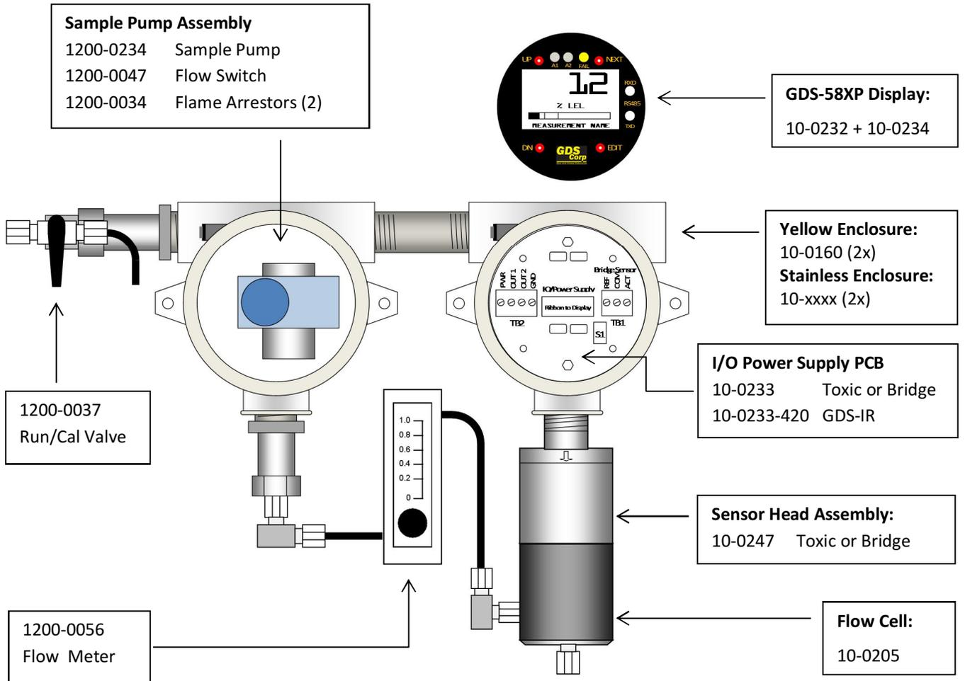
Figure 12-1: GDS-58XP Assembly with Toxic / Bridge Sensor (Spare Parts)
