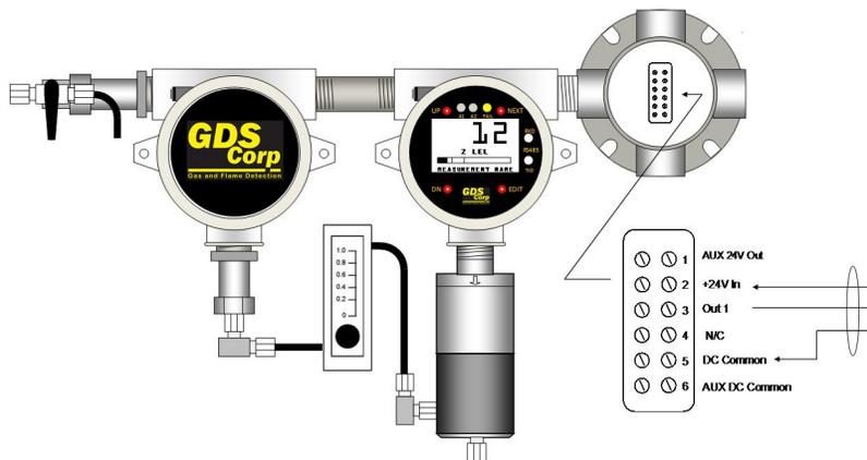
Figure 5-6: GDS-58XP with Analog Wiring Junction Box [RWJB]
