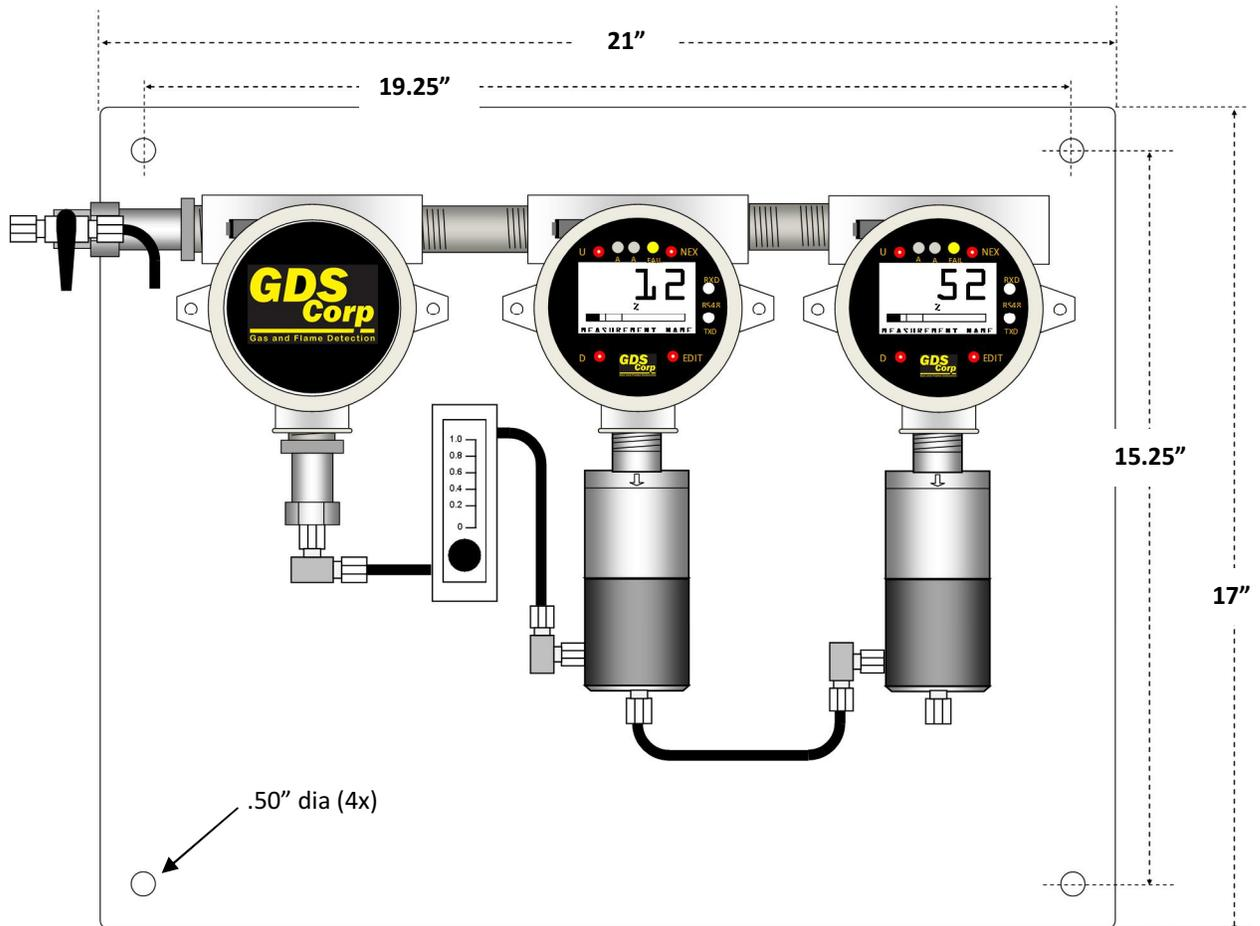
Figure 13-4: GDS-68XP 21" x 17" Mounting Plate Dimensions (AL Enclosures)
