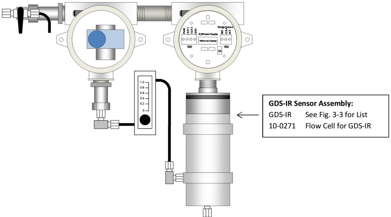
Figure 12-3: GDS-58XP Assembly with GDS-IR (Spare Parts)
