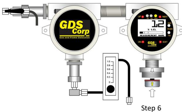
Step 6: Install the new sensor by aligning the arrow on the sensor with the arrow on the sensor head and push straight up.
