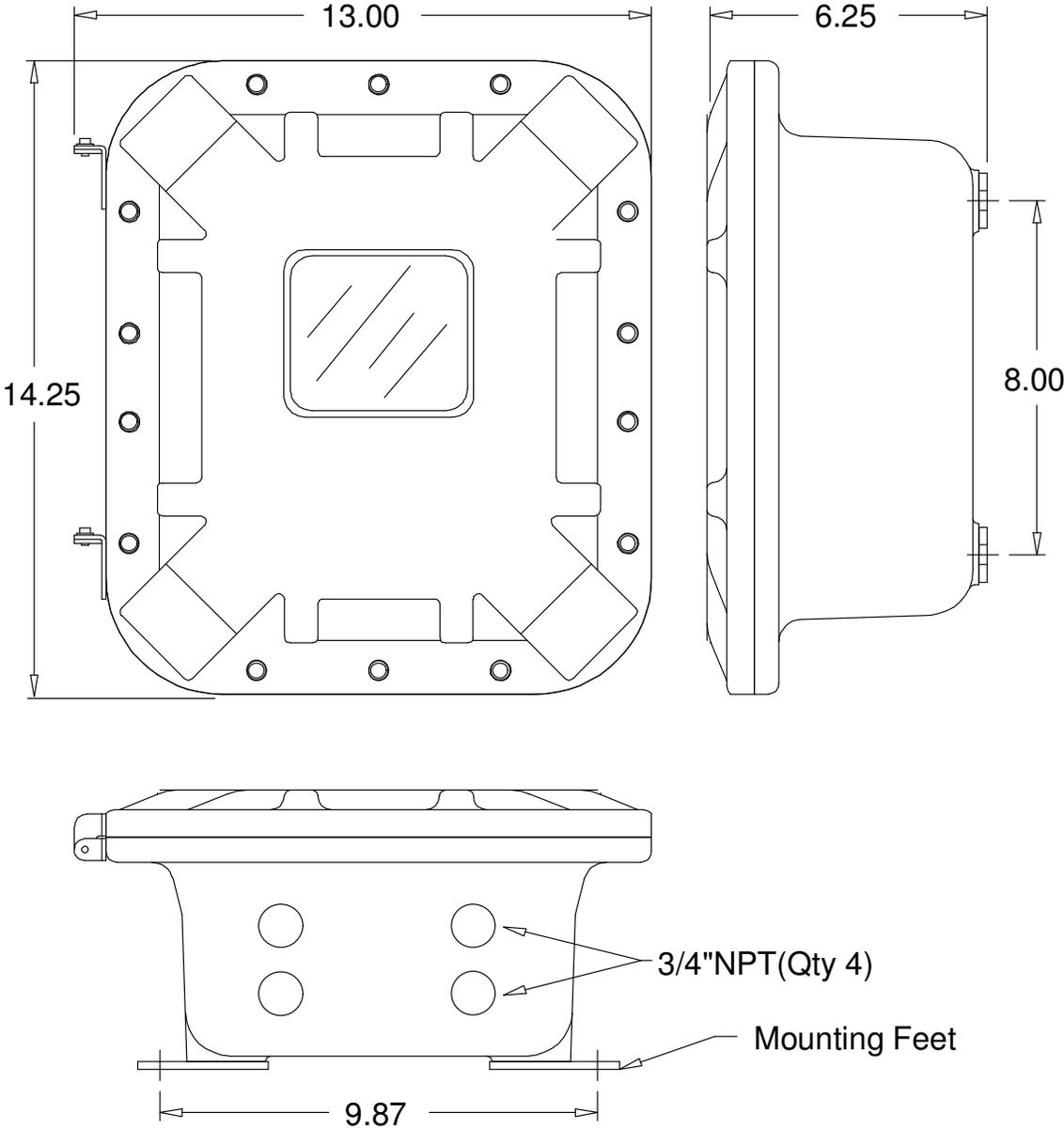
Figure 15-5: NEMA 7 Explosion Proof Enclosure
