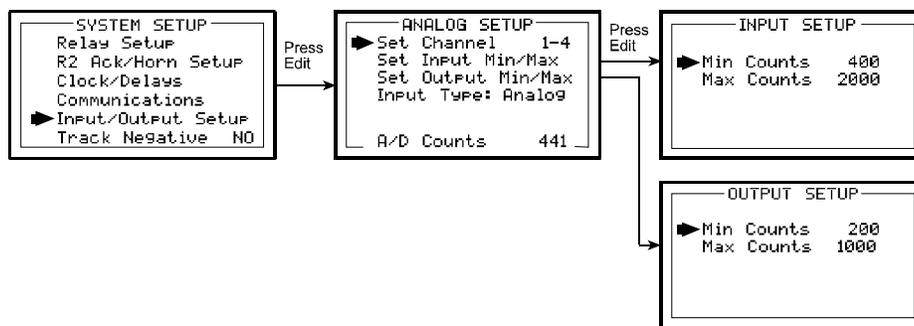
**Figure 11-11: Analog Setup Menu**
