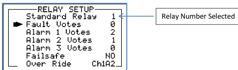
**Figure 11-8: Relay Setup Menu**
