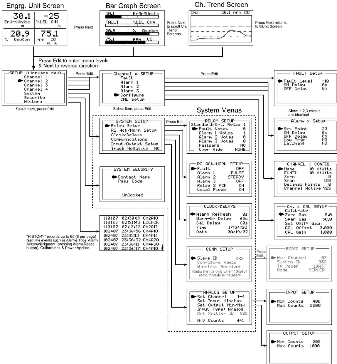
Figure 11-1: C2 Quad Protector Controller Main Menu Tree
