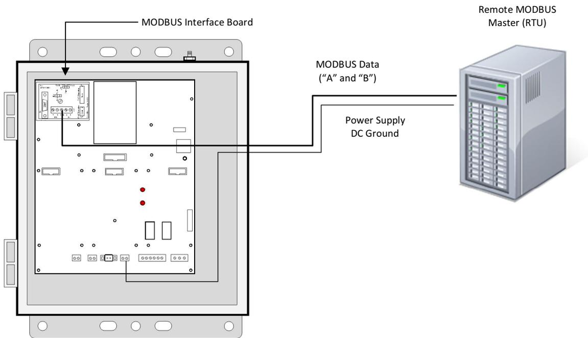
**Figure 7-7: Wired MODBUS Slave Output**
