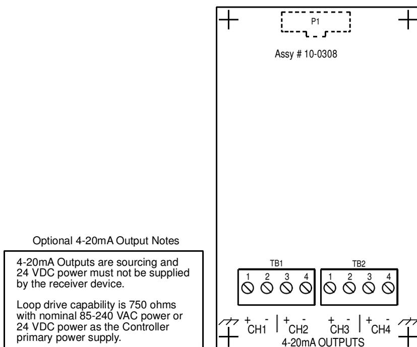
**Figure 6-6: 10-0308 Analog Output Board**
