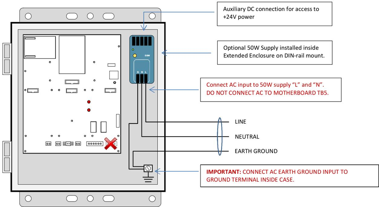
Figure 6-10: Optional 50W Power Supply Wiring
