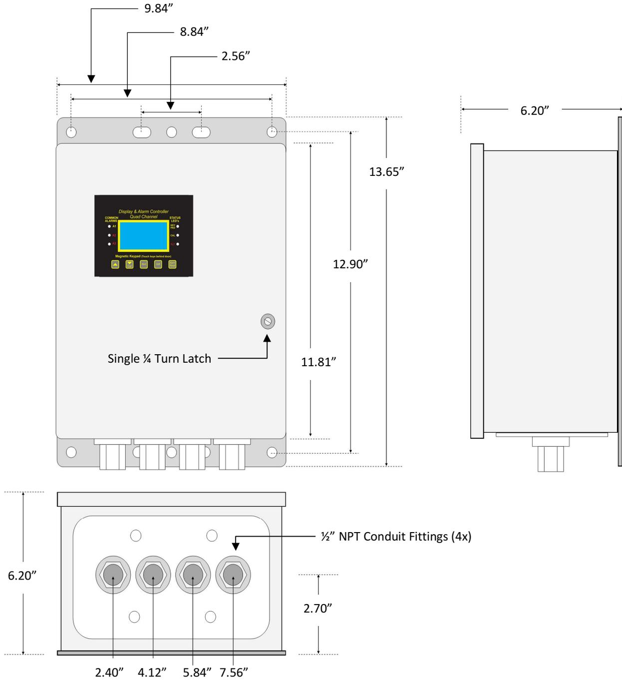
**Figure 15-3: NEMA 4X Painted Steel & Stainless Steel Wall Mount**
