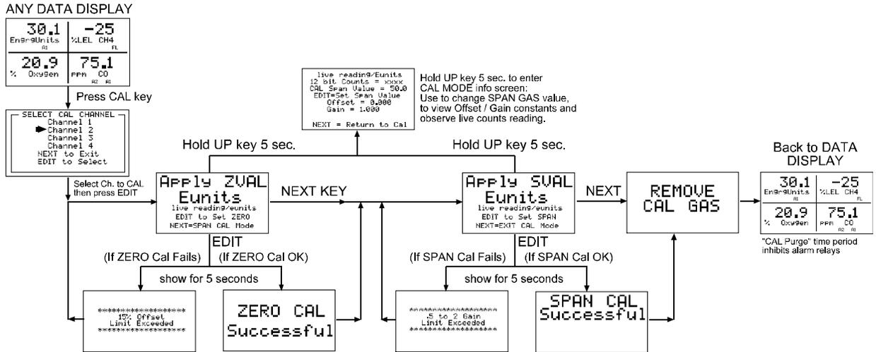
Figure 9-1: C2 Quad Protector Calibration Flowchart
