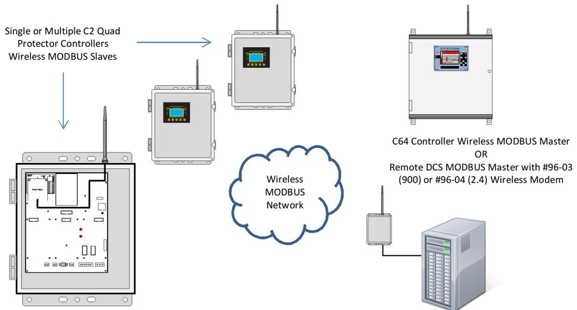
**Figure 7-8: MODBUS Wireless Slave**
