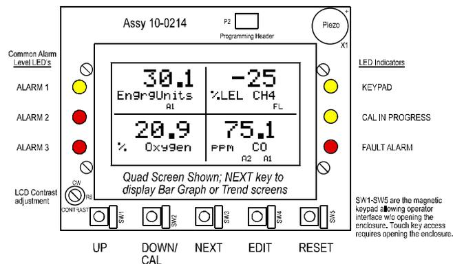
Figure 6-3: Display / CPU Module
