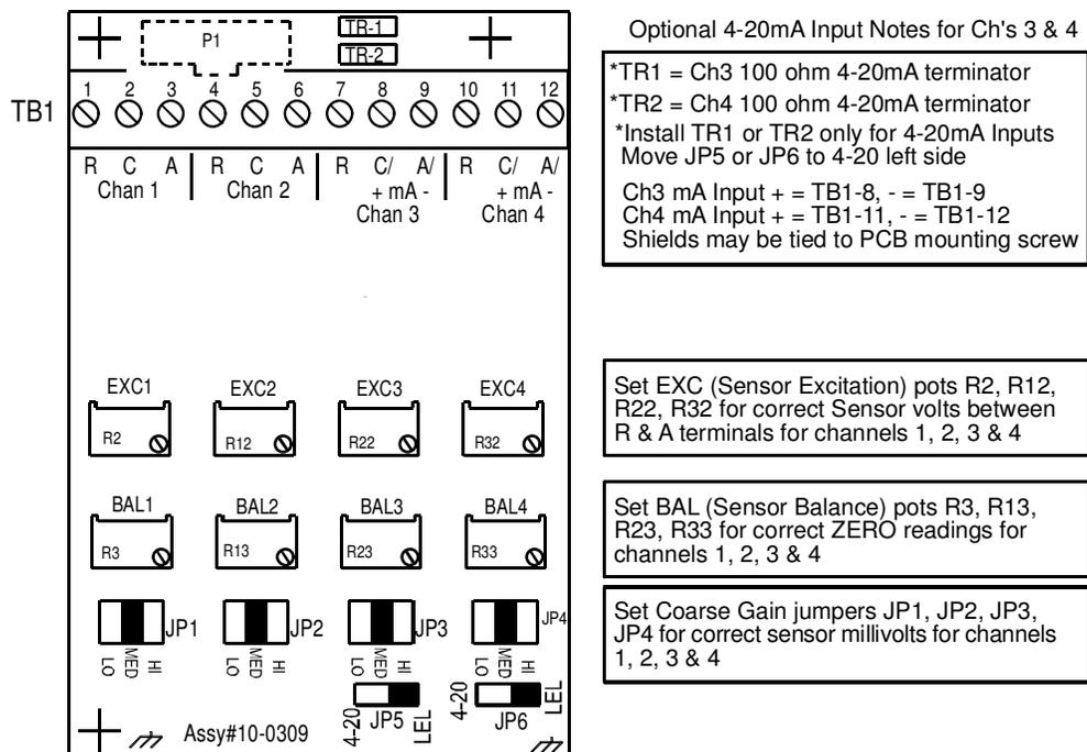
Figure 6-5: 10-0309 Bridge Input Board
