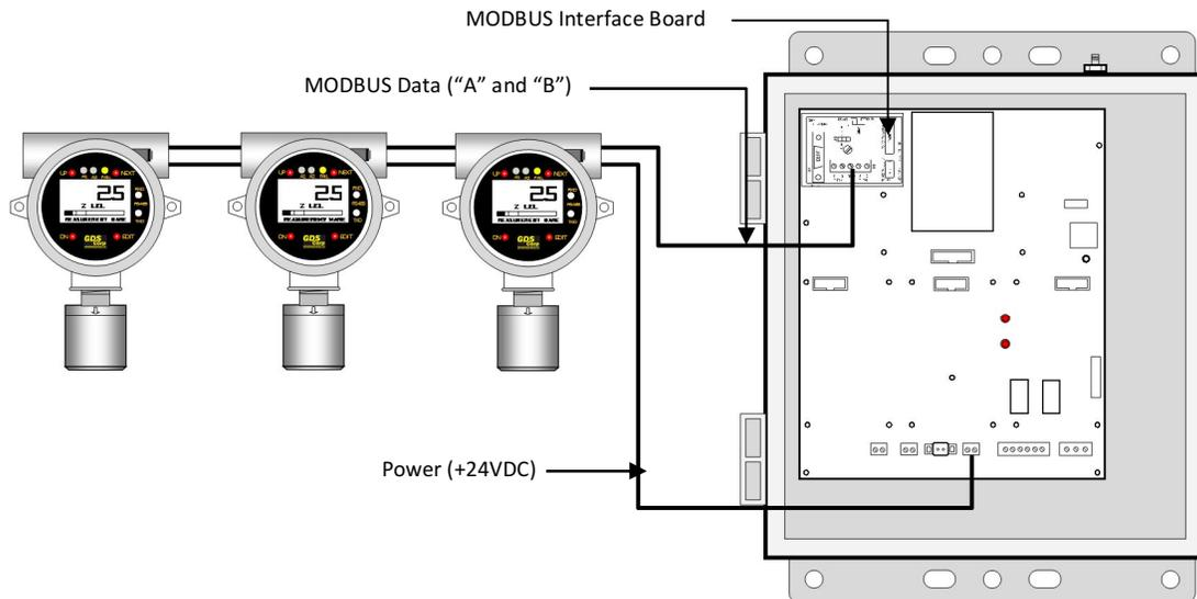
**Figure 7-4: Wired MODBUS Master Input**
