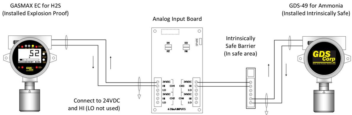
**Figure 7-1: Two-wire Gas Monitors and Transmitters**
