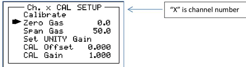
Figure 11-6: Calibration Setup Menu
