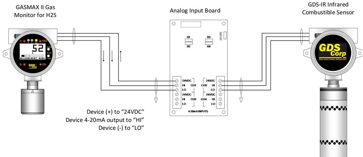
**Figure 7-2: Three-Wire Gas Monitors and Transmitters**
