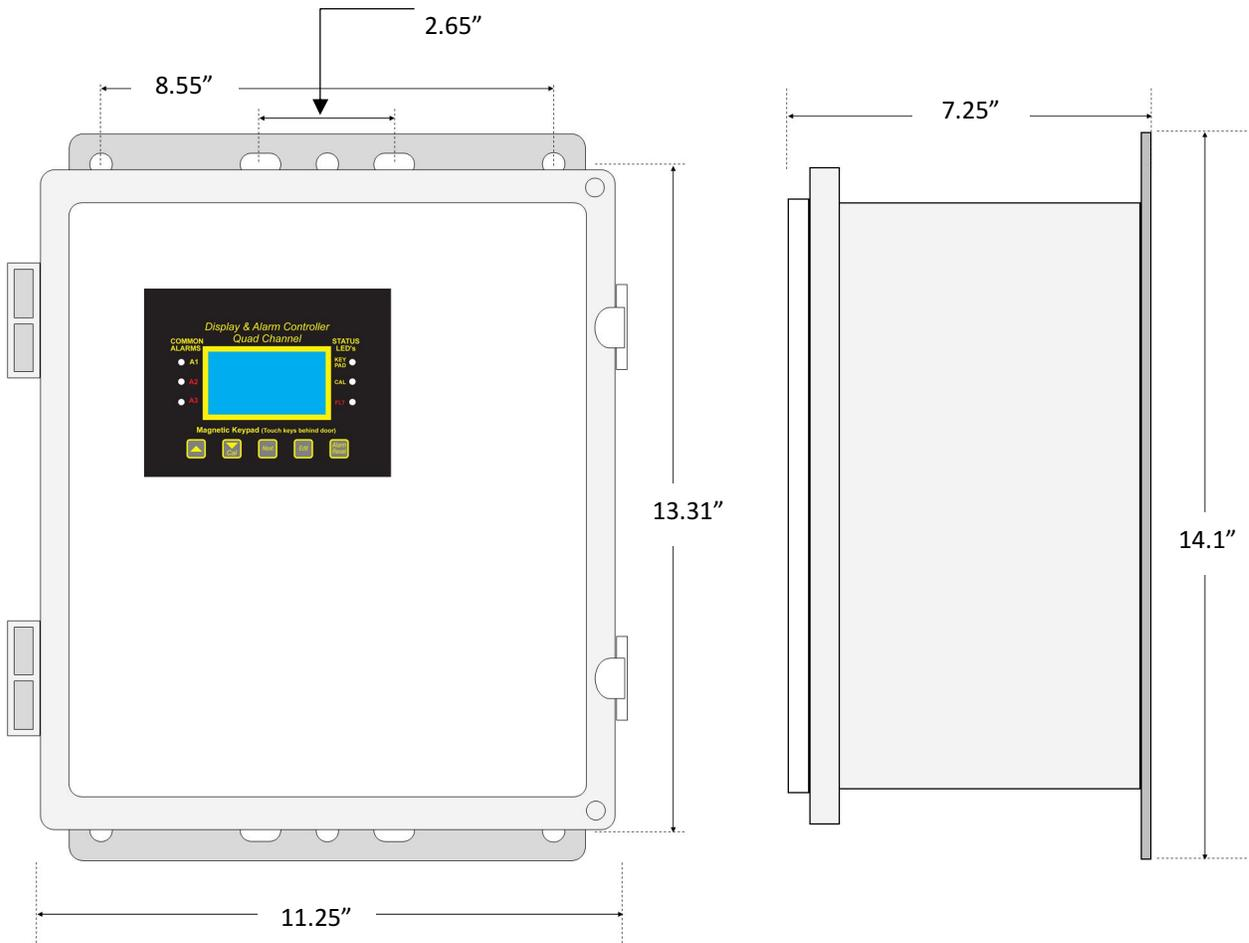
**Figure 15-2: NEMA 4X Polycarbonate Enclosure**
