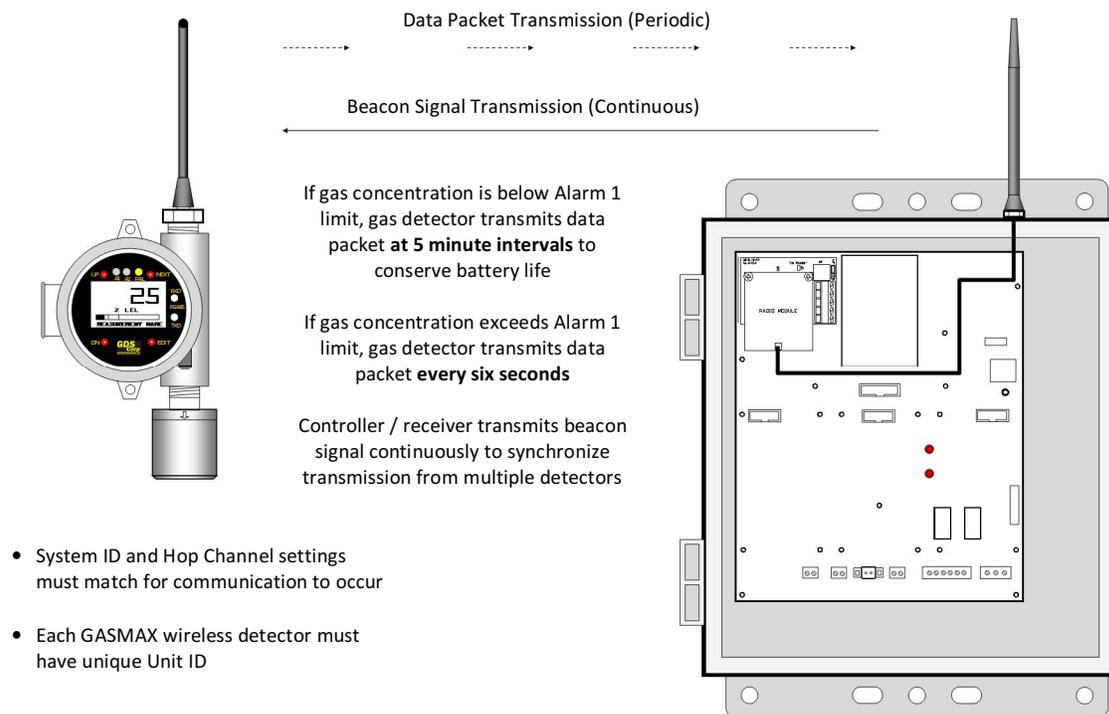
**Figure 7-5: GASMAX ECx and GASMAX TX Wireless Gas Monitors**
