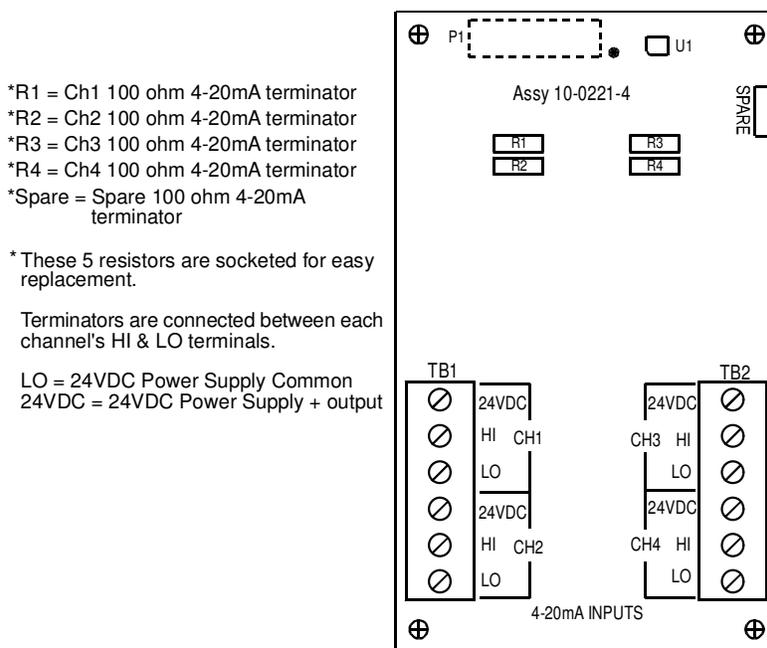
**Figure 6-4: 10-022104 Analog Input Board**
