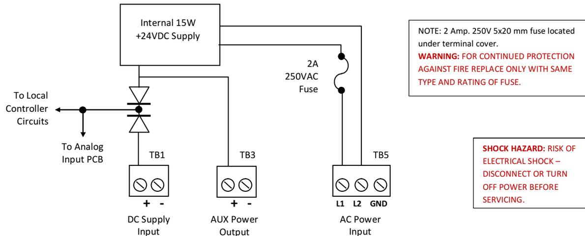
Figure 5-1: Power Supply Input Detail
