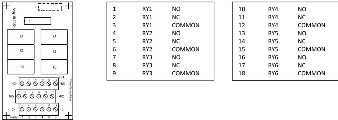
**Figure 7-6: #10-0222 6X Relay Output Board**
