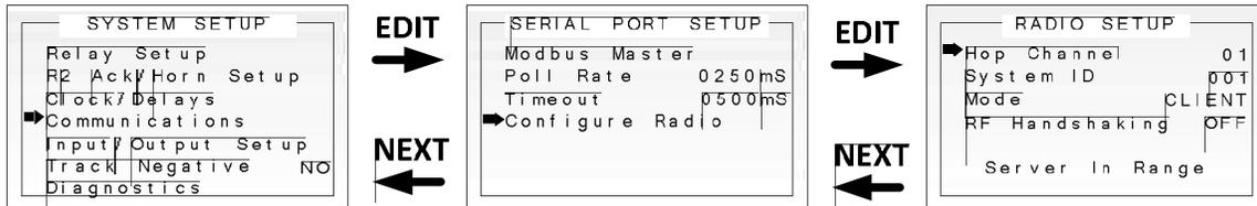
If an RS-485 Serial MODBUS interface card is installed, the following menu items are available:
