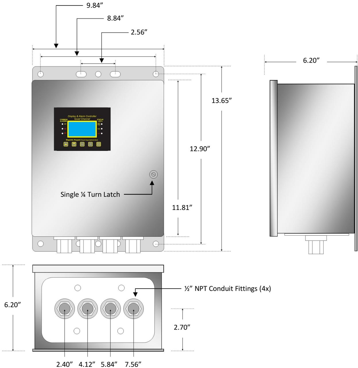
Figure 15-4: NEMA 4X Stainless Steel Enclosure
