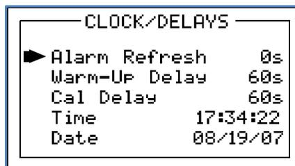
**Figure 11-10: Clock / Delays Menu**
