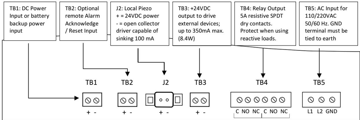
Figure 6-2: Motherboard User Connections Detail
