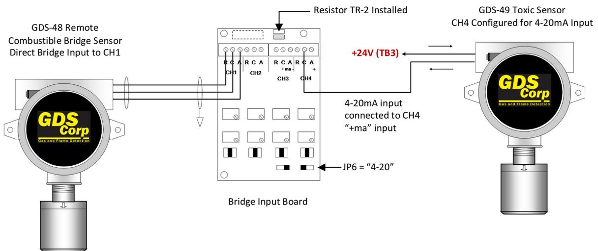
Figure 7-3: Direct Bridge-Type Sensor
