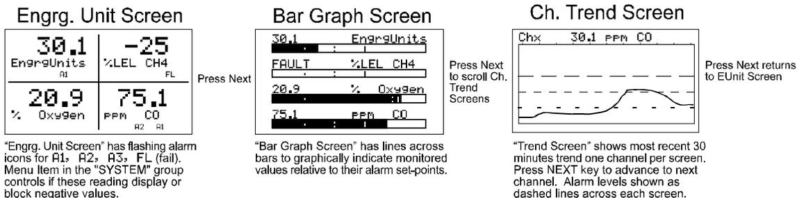
**Figure 8-2: C2 Quad Protector Data Display Screens**
