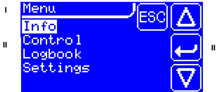
Basic operation is possible with only four buttons which says the same meaning. A pressed button is then displayed. Releasing the button at the same position triggers the function associated with the button.
