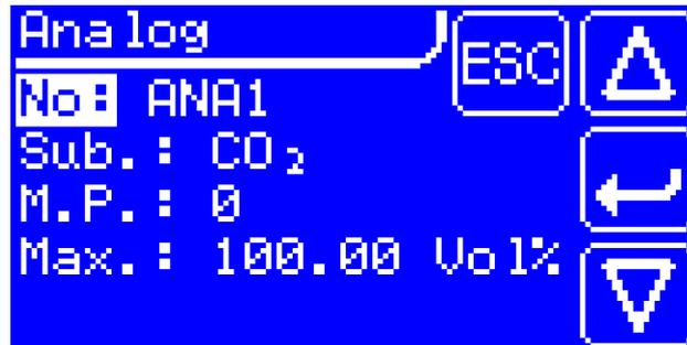
If a number greater than 0 is entered for the measuring point, only the value for this measuring point is updated on the analog output!
