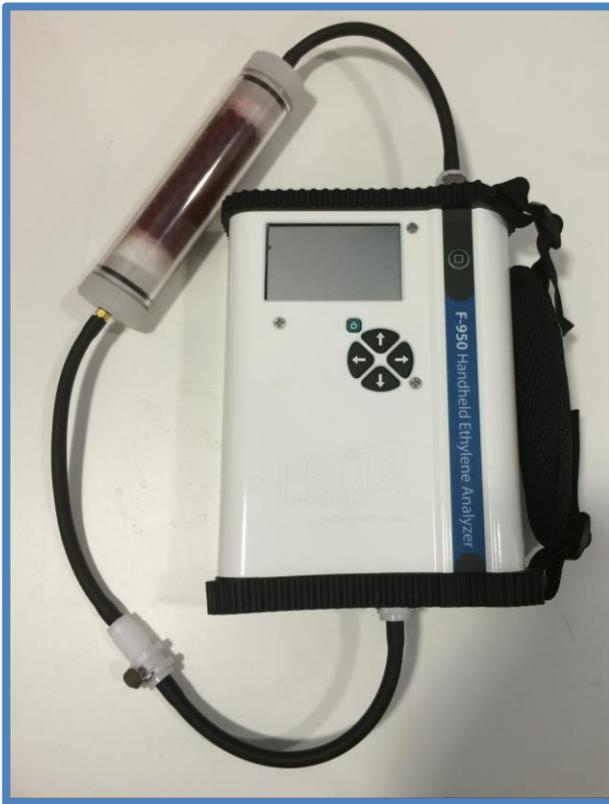
Always store the  $\text{KMnO}_4$  air tight by connecting the ends of the tubing. Replace the cotton ball filters at either end of the external conditioning tube each time the  $\text{KMnO}_4$  is replaced (color indicator turns from purple to brown when it expires).
