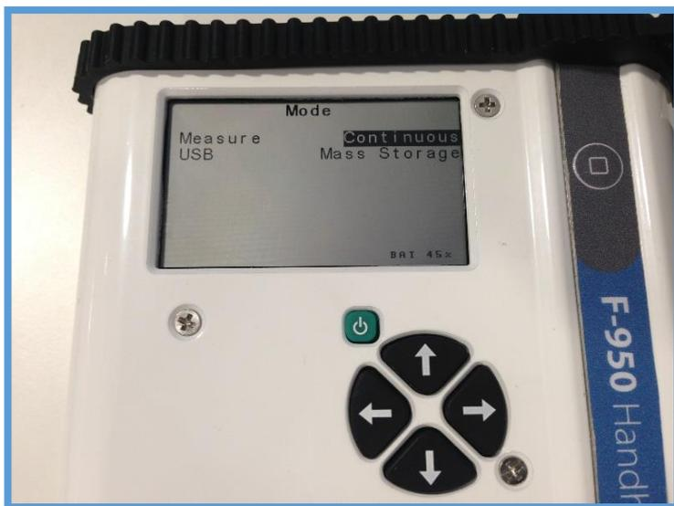
USB mode should be set to Mass Storage. Virtual COM is the other mode, and should only be used to update the firmware if instructed by a Felix Instruments technician.
