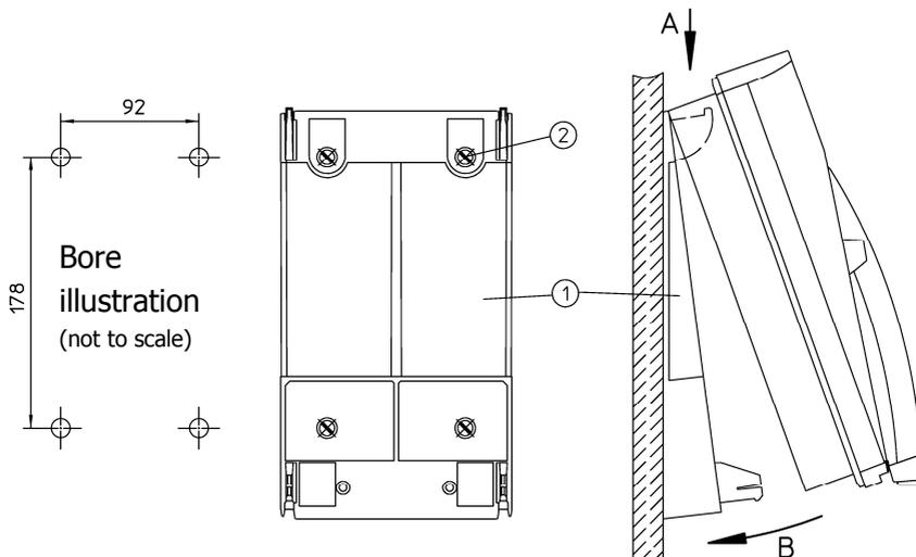
**Figure 4: Mounting on a Wall**
