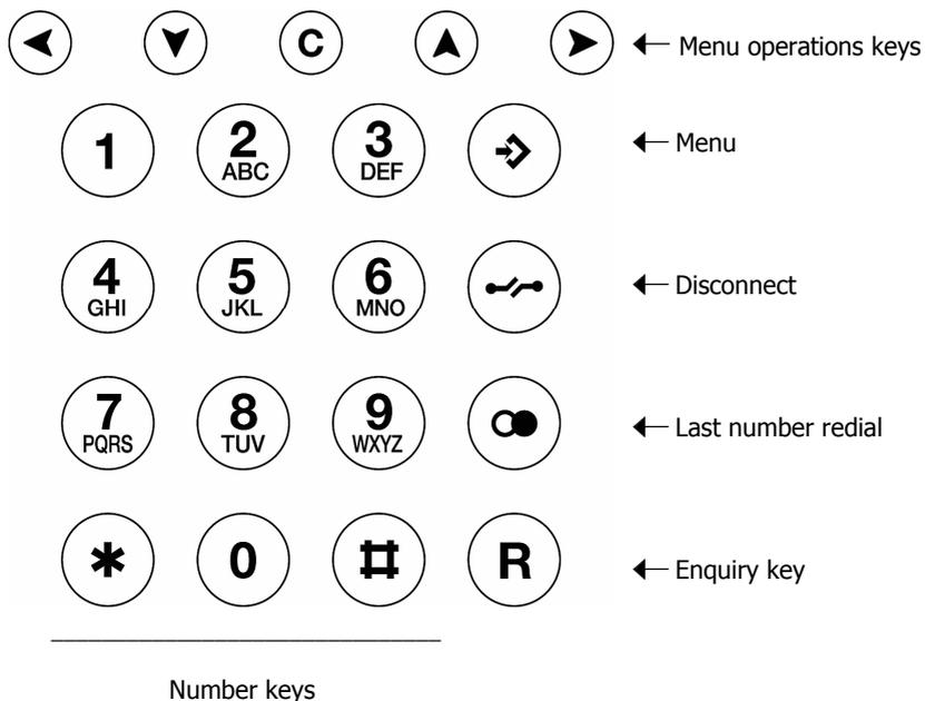
**Figure 1: Keypad of the VoIP-Telephone FernTel IP / IP150**
