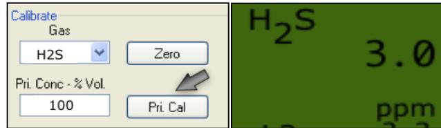
A second gas with a mixture equal to 50% LEL may be used for calibration of span or mid span.
