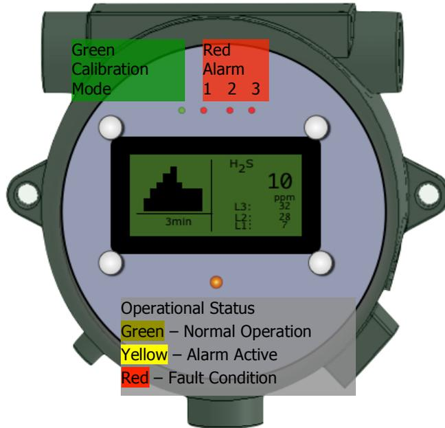
**Figure 3 - SSS-903 LCD Display**
