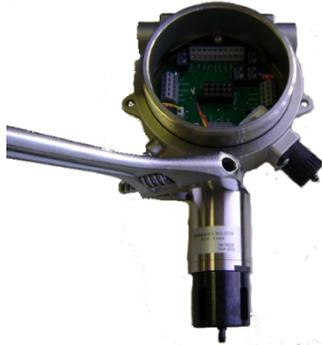
**Figure 13 – Sensor removal**
