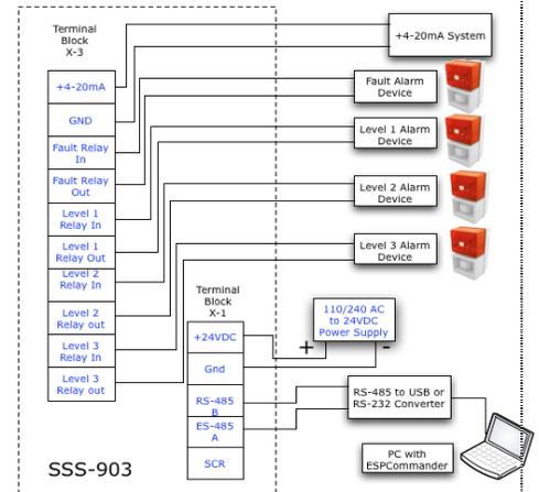
**Figure 27 - Modbus Connection with Analog and Alarm**
