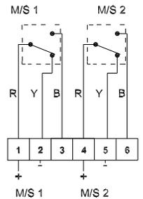
Unit in 'Operated condition' (button pushed in)
