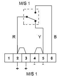
Unit in 'Operated condition' (button pushed in)
