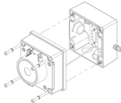
Once the screws are removed the cover will hang down out of the way to gain access to the Ex e terminal block, the internal earth terminal and mounting hole recesses.
