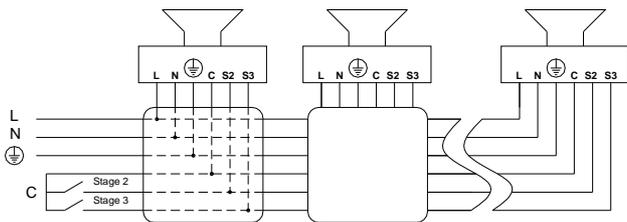
NOTE if the second and third stage wires are not used they must be individually insulated to ensure that cannot make contact to any other wires.
