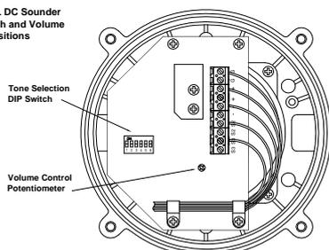
a suitable cable gland. Follow the markings for the terminals on the PCB and install wiring as shown in the diagram below.
