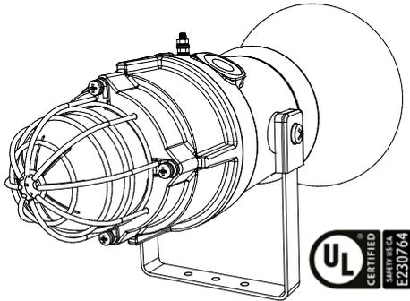
**The D1xC1 & D1xC2 combined alarm horns & strobes are classified by UL as Audible Signaling Appliances for General Signaling and Public Mode Fire Alarm use in Hazardous Locations**
