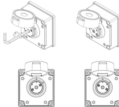
1. On operated unit Twist tool reset button Anticlockwise 55° with special key to reset
