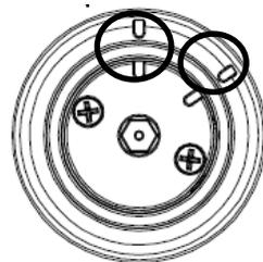
Note: use alignment marks circled to indicate the tool reset buttons status /position.
