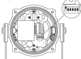
Fig. 9: DIP Switch Location
