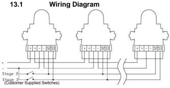
Fig. 6 DC Simplified Block Diagram (negative switching)
