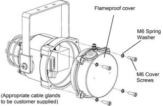
Fig. 2 Accessing the Explosion proof Enclosure.
