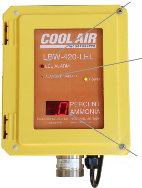
Alarm disabled indication. All relays will be deactivated when this LED is on.
