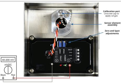
Figure 3: Sensor Output and Zero/span Adjustments
