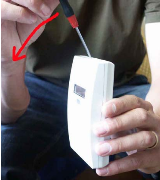
Figure 2. Closed housing seen from the side. The housing is opened by inserting a screw driver and pushing left (to the front side). The locking hooks will then be released.
