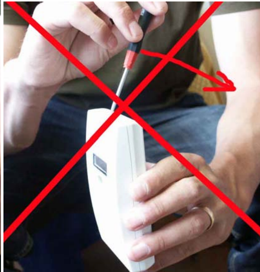
Figure 3. Closed housing seen from the side. Never push to the right. The locking hooks may break and the housing is damaged
