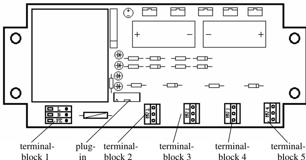
Fig. 4: Power board for magnetic solenoid control
