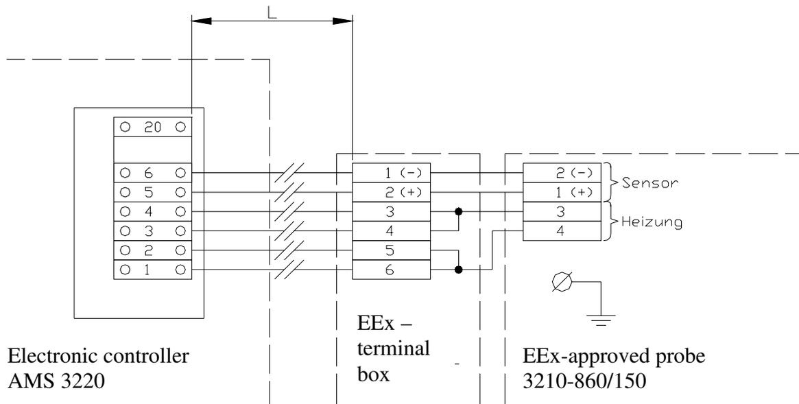
**Fig.3:** Electrical connection between electronic controller AMS 3220 and ZrO<sub>2</sub>-probe 3210-860/150
