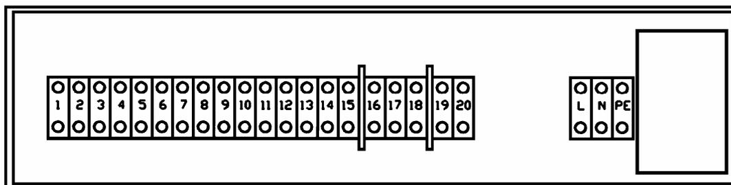
Fig.2: Terminal assignments wall mounted housing (IP65)
