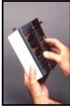
The cell is keyed to ensure proper alignment into the instrument. When installed, the circuit board of the cell should be flat with the bottom of the instrument. Push up on the clear window at the back of the instrument to eject the cell.
